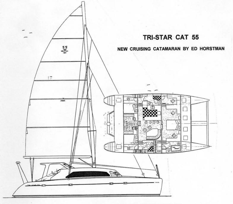
LOA 55'6". LWL 53'. BEAM 32'. DRAFT FIN KEEL 5'3". DRAFT HULL 3'6". DISPLACEMENT 27000#. USEFUL LOAD 12500#. SAIL AREA 1508 FT.SQ.
